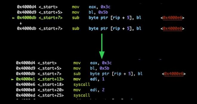
Normally, program code is not modifiable. Compile with gcc -nostdlib -static -Wl,--omagic assembly.S -o bin to make text segment writable.
